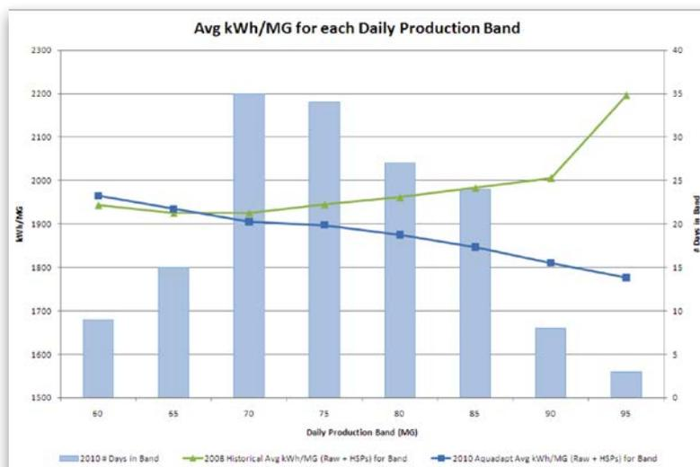
► Figure 1: Two production plants have different energy consumption per MG, as demand increases using the more efficient plant to deliver water leads to big energy and cost savings compared to baseline operation
