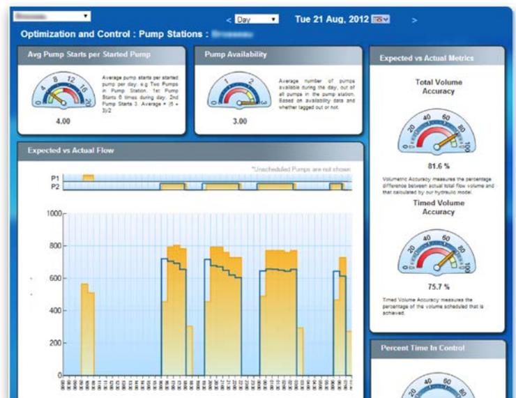
► Figure 2: Aquadapt tracks actual operation, in orange, against scheduled operation in blue, to identify when pumps are manually started, as happened here with Pump 1 at 9:30 am.
