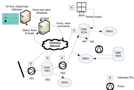
Figure 1. Schematic of a real-time, closed-loop water network optimiser.
