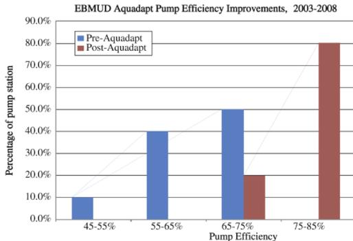
Figure 4. Efficiency improvement in pumps at EBMUD before and after introduction of Aquadapt.
