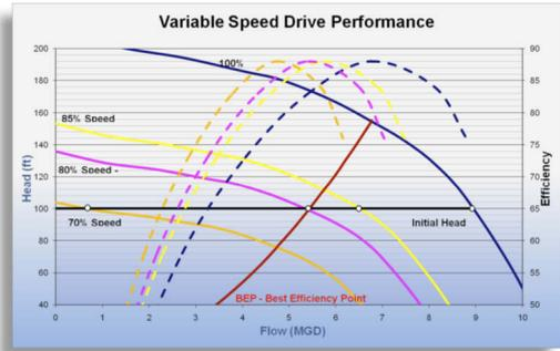
Figure 7. Variable speed pump best efficiency curve.
