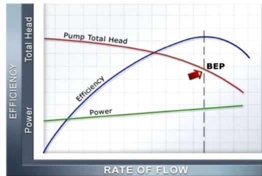
Figure 2. Idealised set of pump curves. Best Efficiency Point ideally at Duty Point.
