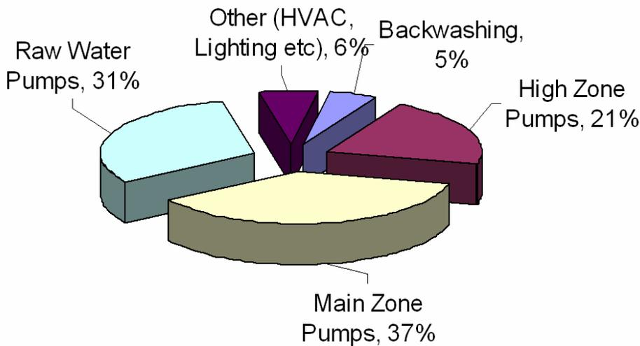
Figure 1: Energy use profile of a large water utility in Maryland
