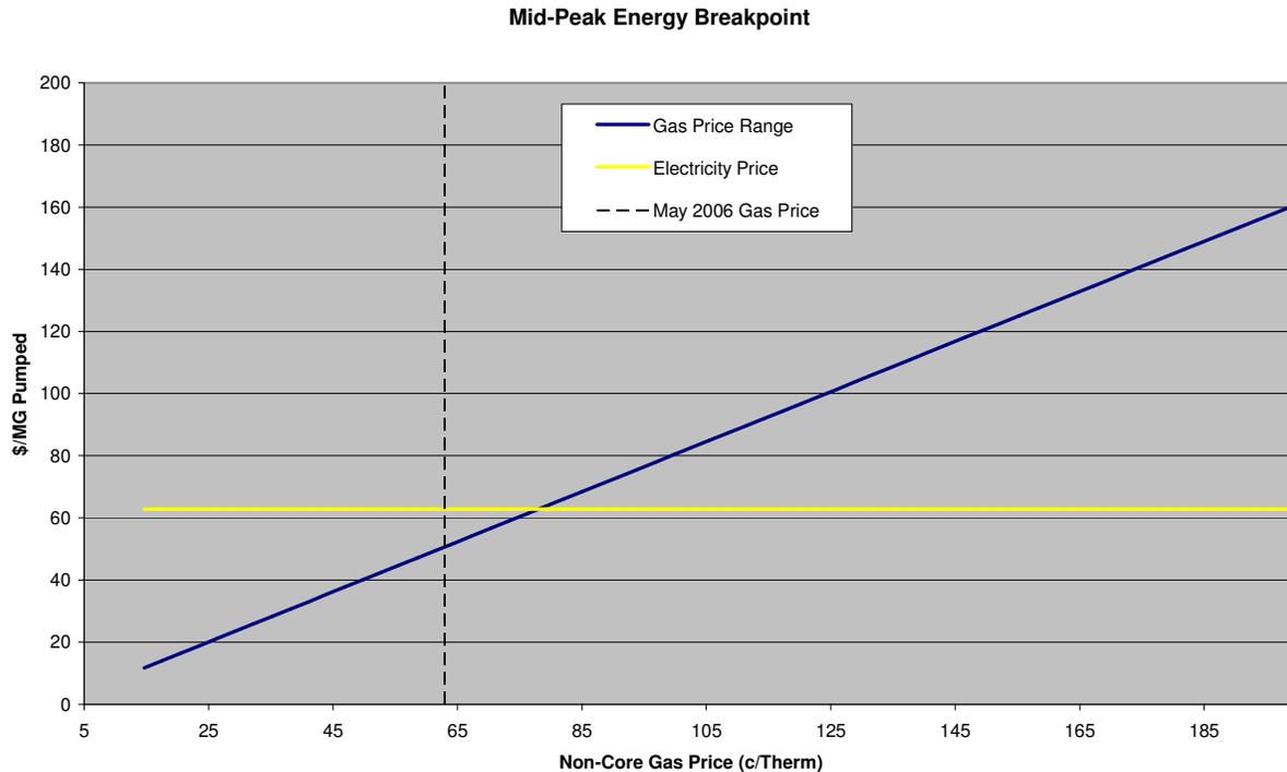
Figure 4 : When gas prices exceeds around 80 cents per Therm, electricity is the cheaper energy source
