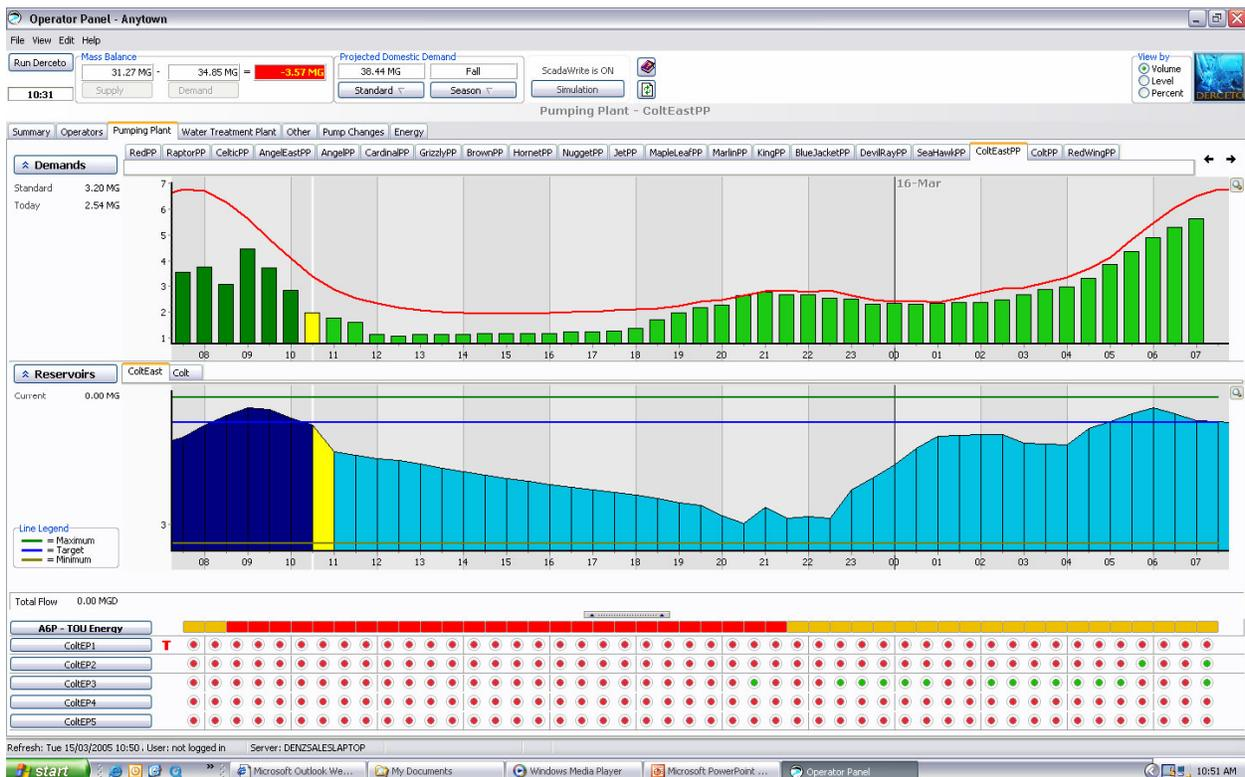
Figure 5: The Derceto operator panel, a thin client GUI which can run across low bandwidth LANs or WANs
